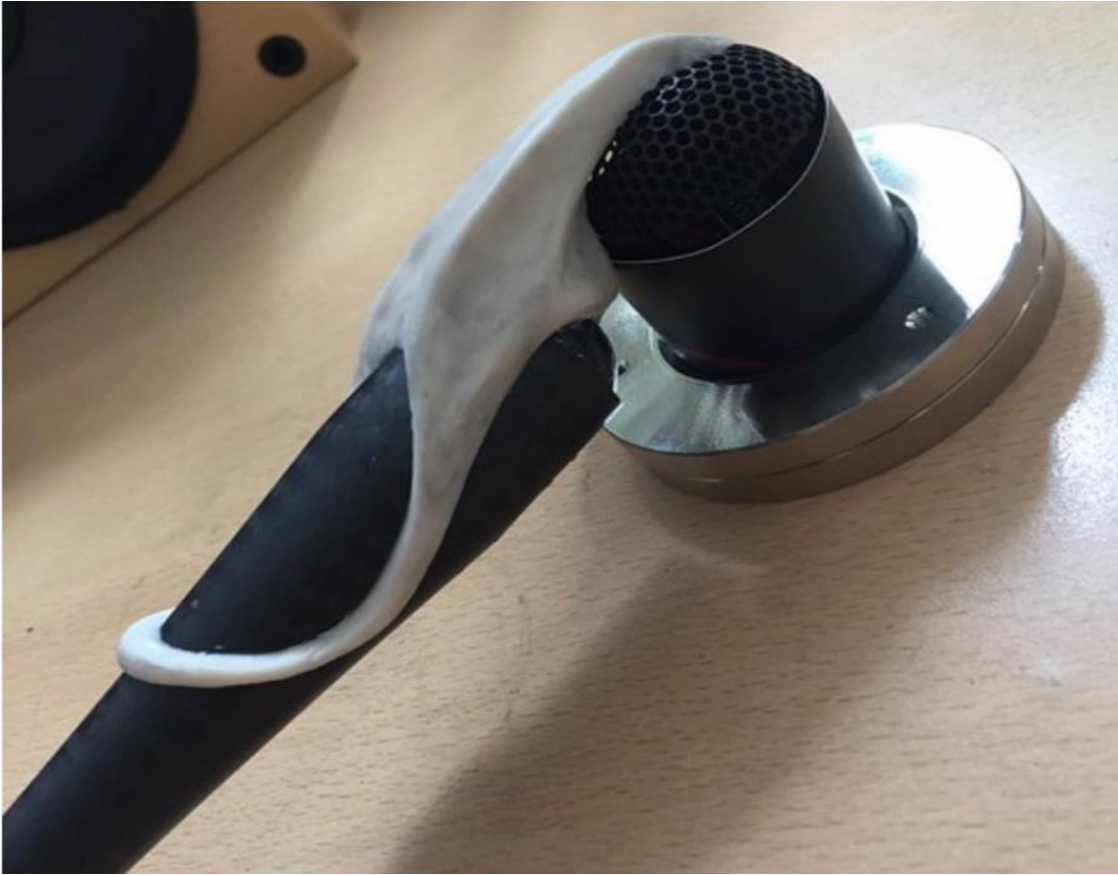
Figure 10: Sculpted by Wilson Benesch Design Director Craig Milnes, this simple wax model was hand-crafted at the outset of the project to visualise basic geometry and mechanical requirements of the titanium counterbalance structure before the team at The University of Sheffield and the AMRC began the additive manufacturing design process.
