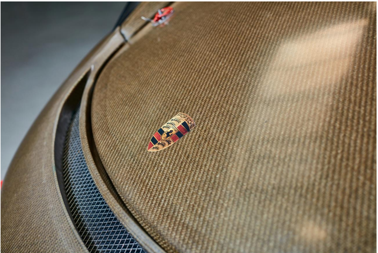
Figure 12: Hemp Fibre Biocomposite body panels used in the chassis of the new Porsche Cayman 718 GT4 CS MR: https://www.bcomp.ch/news/porsche-full-natural-fibre-bodykit/
