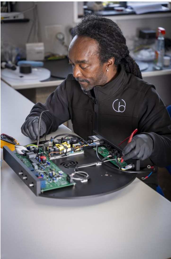
WB: 9 The IGx electronic control boards and class D amplification being tested during construction
