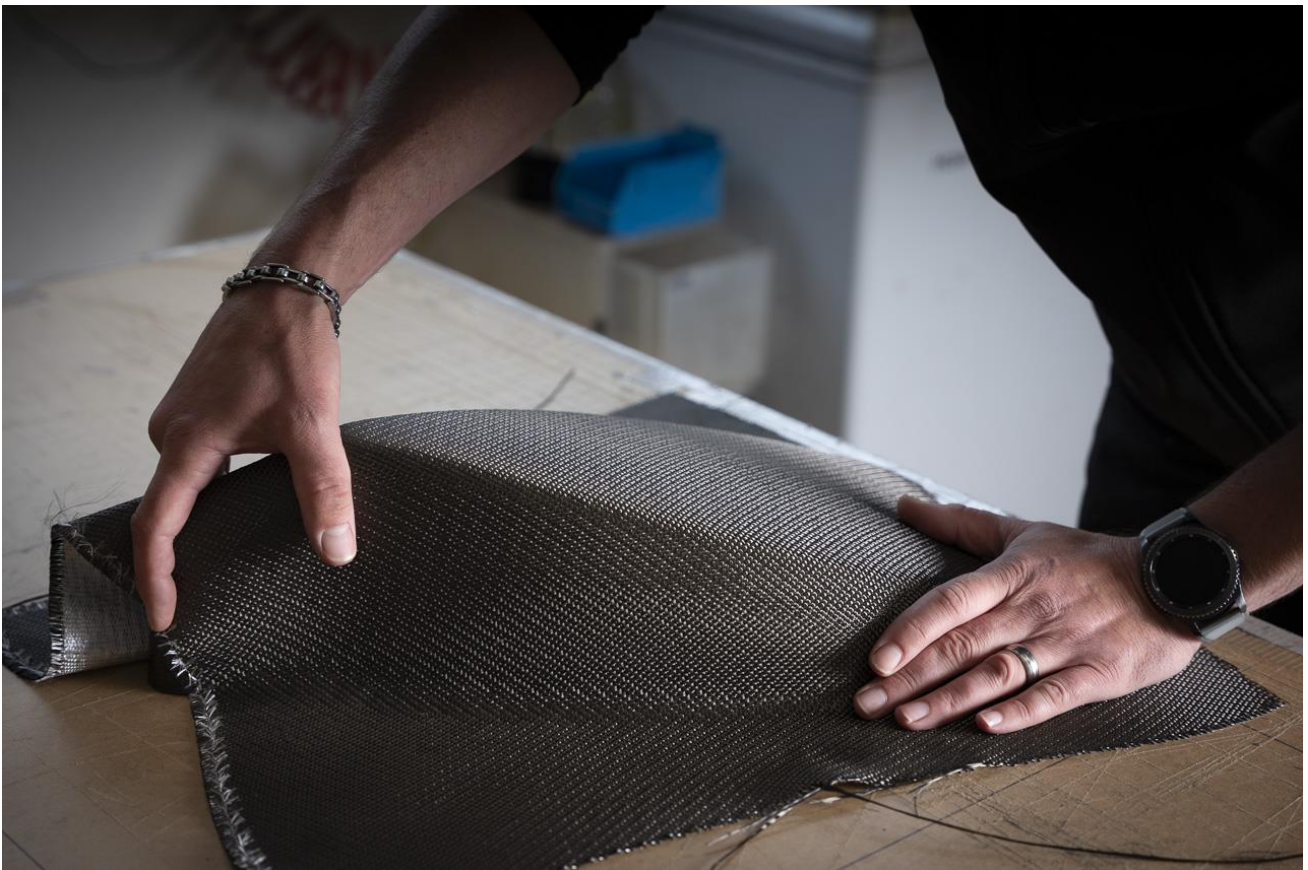
WB: 1 The Carbon Fibre - PET Material that is made specially for Wilson Benesch is also used in the carbon fibre tops that are used in the company's reference loudspeaker line. Seen here a technician forms the top of the Endeavour 3zero loudspeaker.
