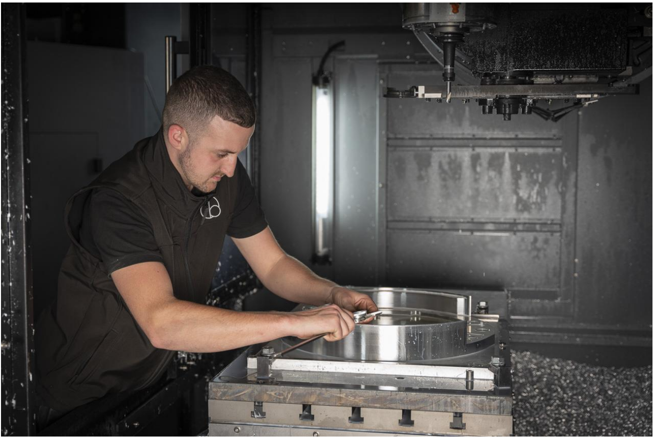
WB: 10 The IGx base being machined in the Wilson Benesch CNC Suite at Falcon House
