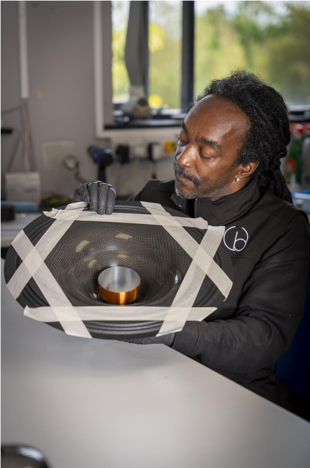
WB: 8 The IGx 18" Carbon Fibre - PET diaphragm in production with the cambric fabric surround and top voice coil shown
