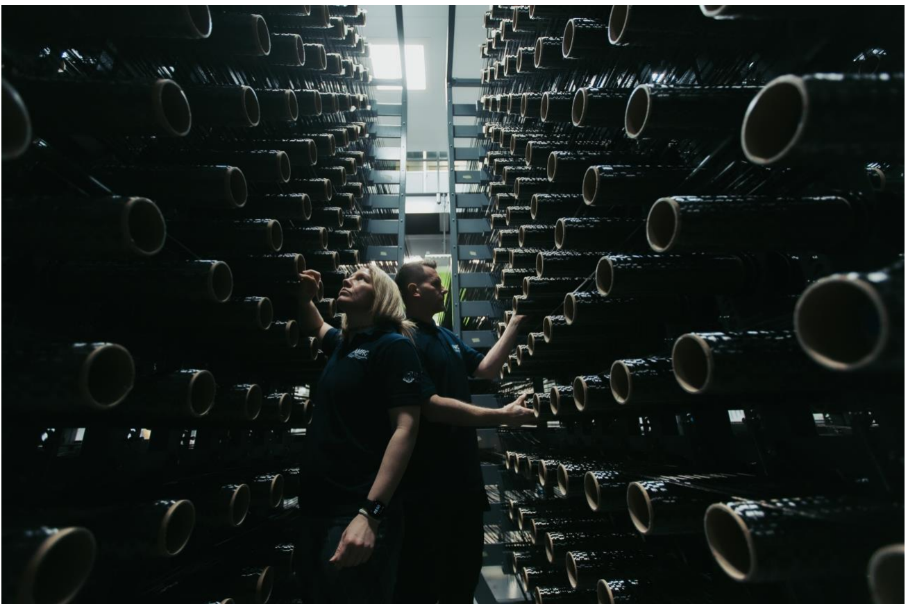
WB: 3 The Carbon Fibre Spools that feed the weaving machine to create carbon fibre fabric
