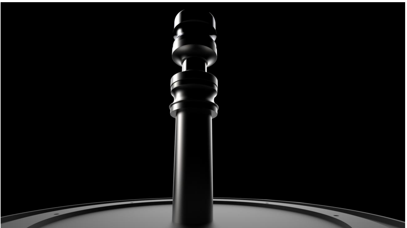
WB: 7 With the coils removed the two large Neodymium Rare Earth Magnets can be observed residing around the central steel Core
